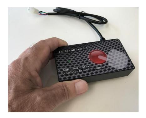
Using a proximity sensor, BDS created the perfect button for the system. It senses a person's finger and has no moving parts for a very, very long life. Integrated with a transmitter, the buttons can signal the controller wirelessly for easier installation. And dedicated power means no batteries are required.
